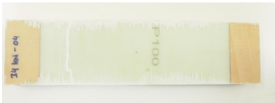
Figure 16: Representative failure of the specimens tested at 34.07 kN and 3.6 kW/m 2
