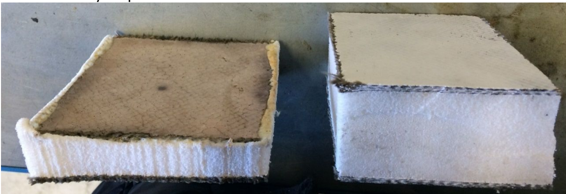
Figure 1: Sandwich made with geopolymer skin and DIAB Divinycell P100 core before and after an ignition test under the cone calorimeter at 20 kW/m 2 .
