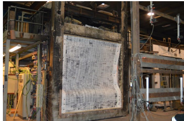
The FRP bulkhead collapsed after 82 minutes of exposure to ISO 834-1.
