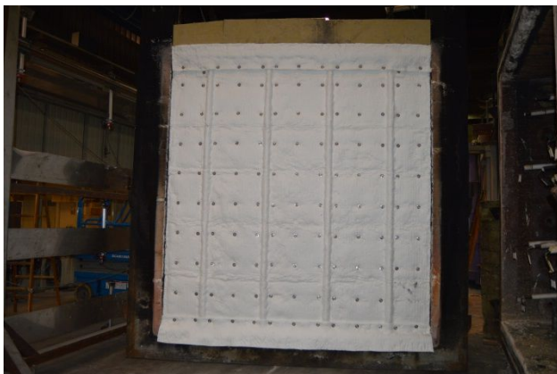
The exposed face of the steel bulkhead (insulated) before the fire test.
