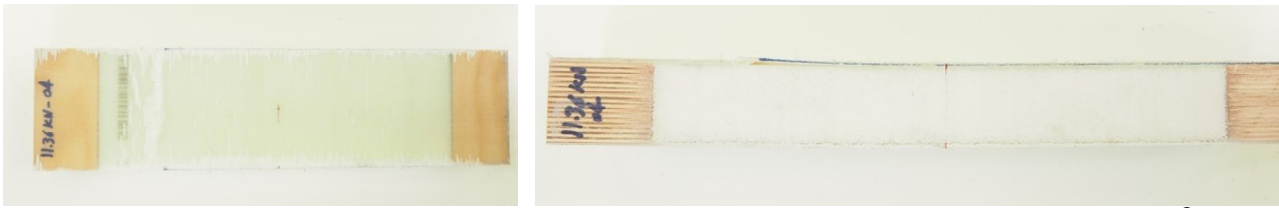
Figure 18: Representative failure of the specimens tested at 11.36 kN and 3.6 kW/m 2
