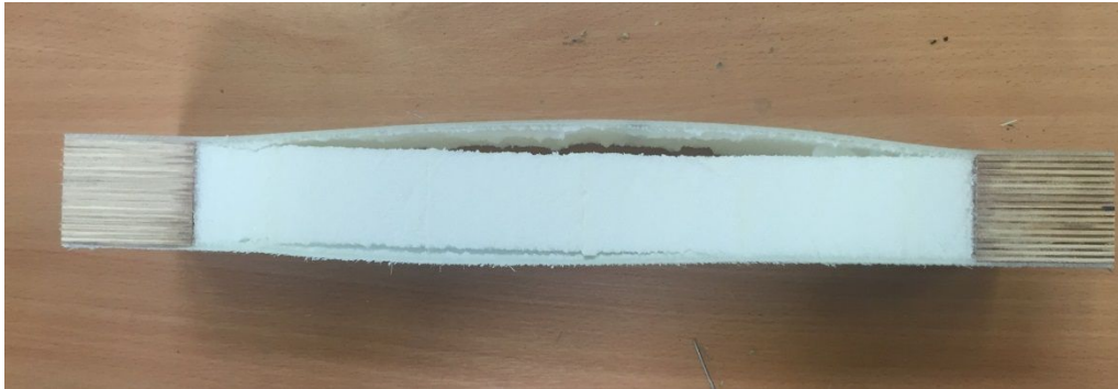
Figure 12: Typical failure mode of the reference specimens
