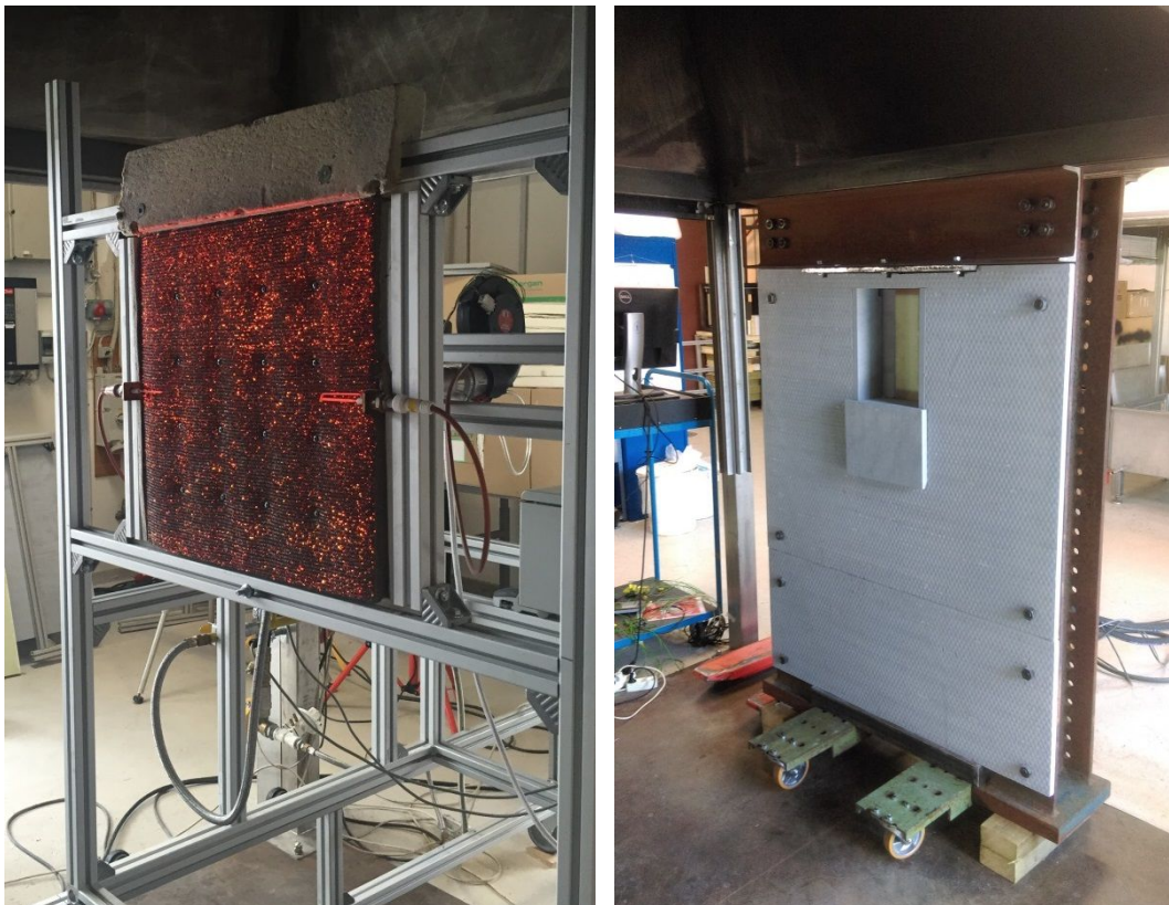
Figure 1: Burner (left) and insulated loading rig (right)
