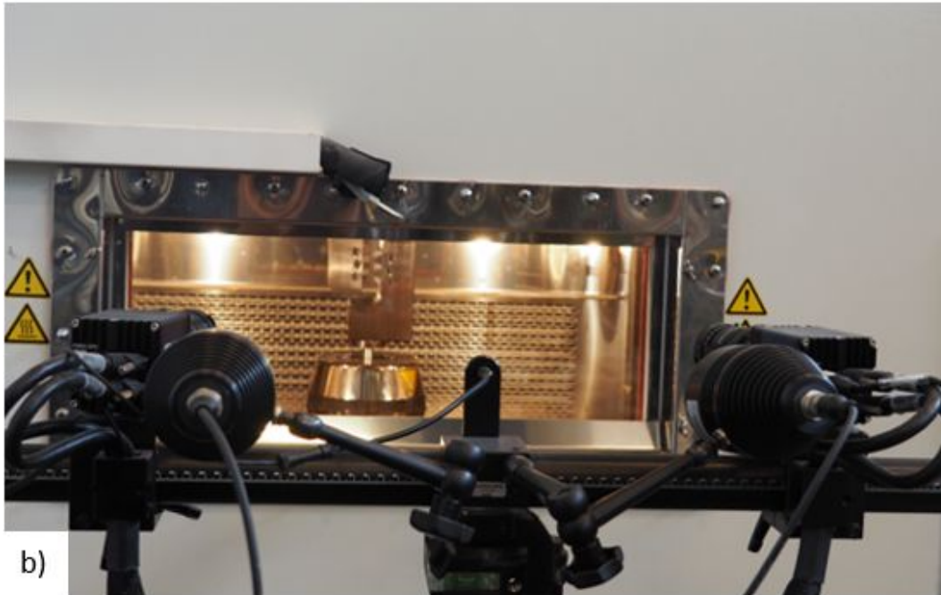
Figure 8. Experimental setup a) v-notched shear properties test b) DIC cameras
