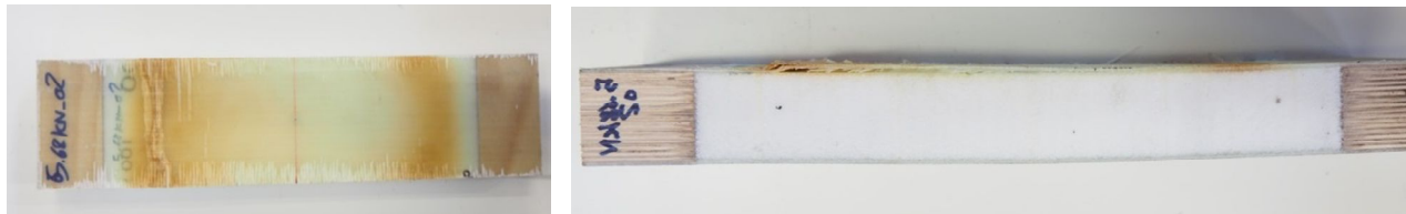
Figure 19: Representative failure of the specimens tested at 5.68 kN and 3.6 kW
