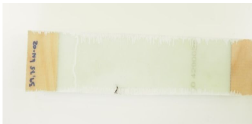
Figure 15: Representative failure of the specimens tested at 39.75 kN and 3.6 kW/m 2
