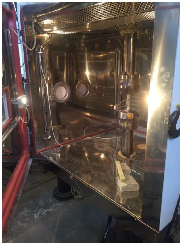
Figure 1. Environmental chamber mounted to the testing machine
