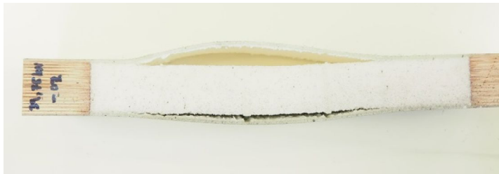
Figure 15: Representative failure of the specimens tested at 39.75 kN and 3.6 kW/m 2
