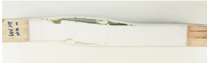
Figure 16: Representative failure of the specimens tested at 34.07 kN and 3.6 kW/m 2
